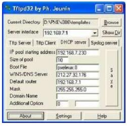
Configure your **DHCP Server** here. Booting with PXE is not possible unless you define it. A common network configuration is to have addresses like 192.168.0.x with 192.168.0.1 as the router (often a workstation connected both to the internet, both to the LAN, and sharing the internet connection on the LAN).
